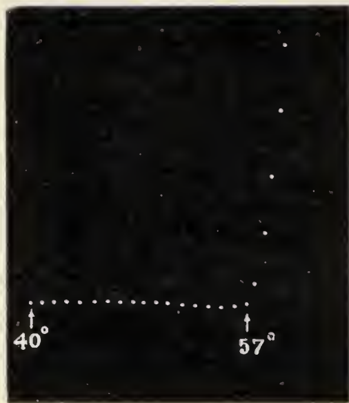
FIG. 135. Record of living tissue balanced by dead. Sudden increase in weight at 57^{\circ} C.
